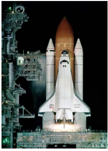
The two auxiliary Solid Rocket Boosters are clearly visible, on each side of the rocket
