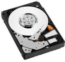
The 2.5-inch VelociRaptor has a rated speed of 10k RPM Western Digital
