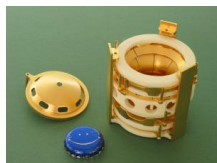
Image of a LEBIT ion trap (the bottle cap in the lower part of the image is for scale) NSCL
