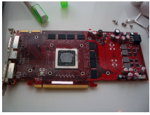
The HD 4850 graphics card stripped down of its cooling system bit-tech
