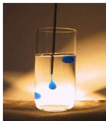
This image shows ionic liquids (the blue globules) in a beaker of mineral oil John Wilkes
