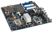
The Skulltrail, the only non-server platform to sport two processors Hot Hardware
