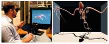
(Left) An artist uses Drawing on Air: a stereoscopic desktop display, stylus and tracking device. (Right) An image of a 3D bat skeleton made with the system Daniel Keefe and col.
