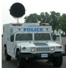
LRAD sonic weapon mounted on an armored Humvee belonging to the NYPD American Technology Corporation (ATCO)
