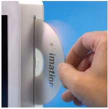
The slot-loading drive is intended for use with standard disks only Imation
