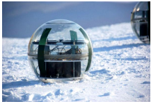
GPS buoys deployed during the campaign to monitor the ice movement ESA
