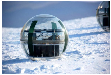
GPS buoys deployed during the campaign to monitor the ice movement ESA
