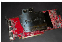
Diamond Multimedia equips AMD's flagship card with Koolance liquid cooling solution Diamond
